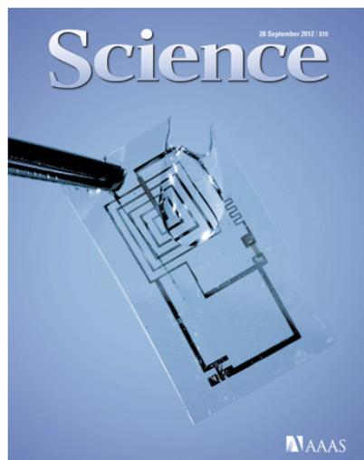
Physicians and environmentalists alike could soon be using a new class of electronic devices: small, robust and high performance, yet also biocompatible and capable of dissolving completely in water or bodily fluids.
