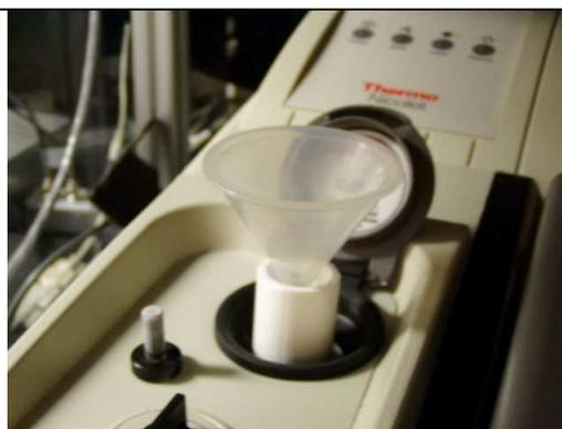
(2) Filling the detector with liquid N<sub>2</sub>
